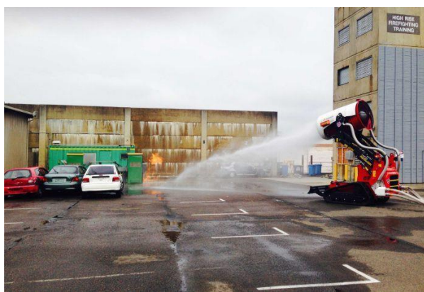
1 - PHOTO: The TAF 20 firefighting robot can blast water up to 90 metres and spray water mist or foam for 60 metres. ( ABC News: Brigid Glanville )
